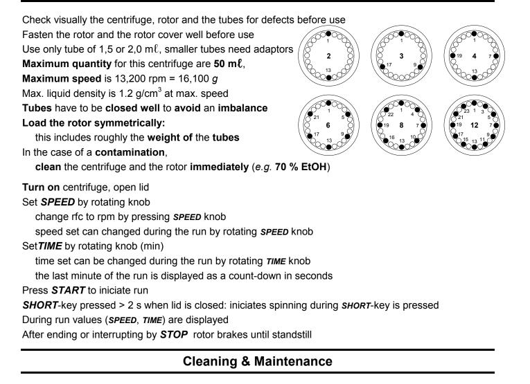
**Dry condensation water** within the rotor chamber. Keep the lid open to dry the rotor chamber **Clean** and **disinfect** the centrifuge and rotors (& rotor bores) **monthly** with neutral detergents Clean rubber seals well with water and put **glycerol** to **protect** the **seals**
